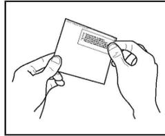
Before using the Jasic JH-HD helmet for the first time, the protective films must be removed from the front spatter lens. The films cannot be removed from the front spatter lens with the lens in place. Please follow the instructions below to remove the spatter lens.
