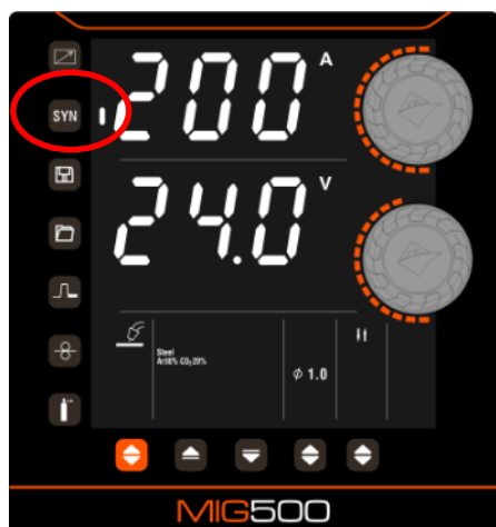
EM-350S & EM-500S Power Source Control Panel
