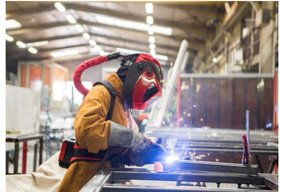
An example of personal fume protection
