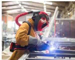
An example of personal fume protection
