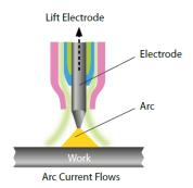
The Jasic Arc range allows the tungsten to be in direct contact with the work piece with minimal current so as not to leave tungsten deposits. Once contact has been made the tungsten can then be lifted away 2-4mm from the work piece and the welding arc is then established.
