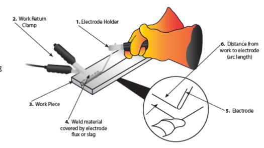
Welding current will flow in the circuit as soon as the electrode contacts the work piece. The welder should always ensure a good connection of the work clamp. The nearer the clamp is placed to the welding area the better.
