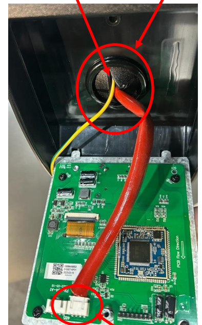
Control PCB Socket CN6 (I)
