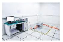
**Conducted Emission Disturbance Testing**
