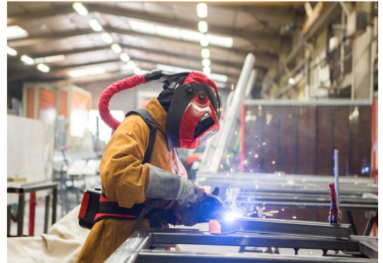
An example of personal fume protection
