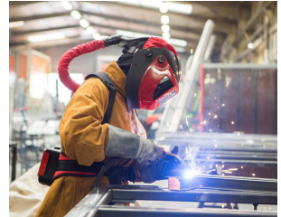
An example of personal fume protection
